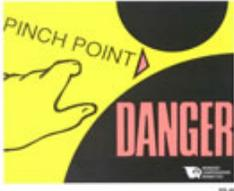
When two rotating mechanical parts move together with at least one of the parts moving in a circle, a pinch point hazard is created. Agricultural equipment and machinery frequently have pinch point hazards including gear, belt, and chain drives, sprockets, conveyors, and feed rolls. California Code of Regulations (CCR) addresses pinch points under Title 8, Sections 3440, 3999, 4002, 4070, and 4075.
